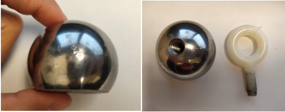
Figure 3- 9. Configuration of the Created Steel Ball and Plastic Hook Connection
